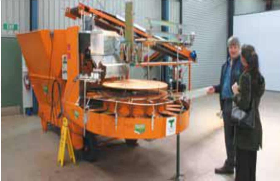
Automatic pot filling machine fill up, fertilized and potted exactly 4800 pots per day at South Gippsland Victoria
